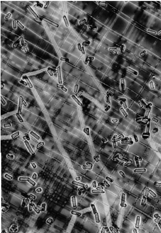
Figure 7. Photomicrograph of a TN cell with dye polarizing–alignment layers while 6 V is applied; note the dual domain structure.
